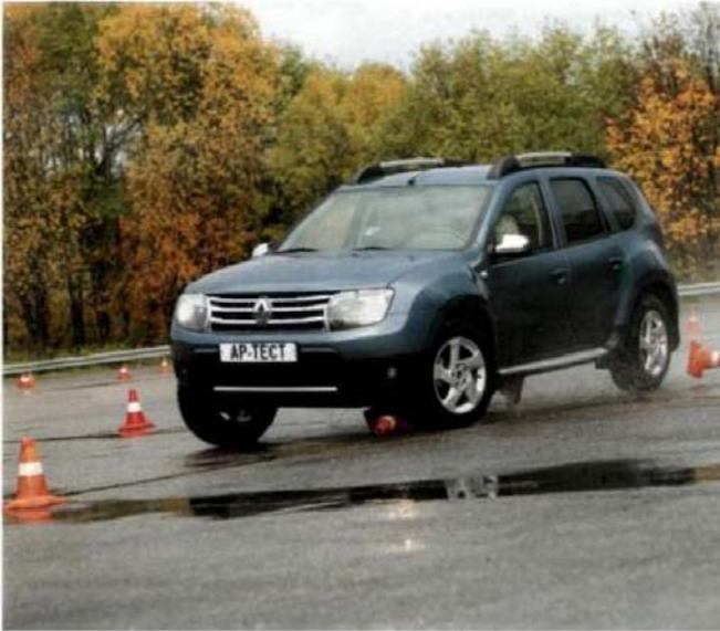
*The speed was too high on entering the turn and the car skidded and knocked over a cone. But we changed the tires and the Duster easily made the turn at the same speed.*
