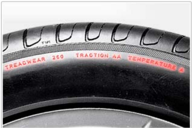
**TRACTION:** The traction grades, from highest to lowest, are AA, A, B, and C. These grades represent the tyre's ability to stop on wet roads as measured under controlled conditions on specified government test surfaces of asphalt and concrete. A tyre marked C may have poor traction performance. Caution: the traction grade assigned to the tyre is based on straight-ahead braking traction tests, and does not include acceleration, cornering, aquaplaning, or peak traction characteristics.
