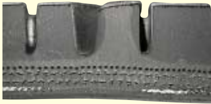
Section of a tread with conductive inserts.
